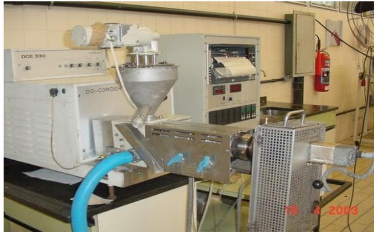
**Figura 3.** Extrusor de rosca simples Brabender 19/20DN
