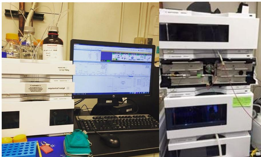
**Figura 16** - UPLC/ESI-HR-Q-TOFMS, 6500 Series, Agilent.
