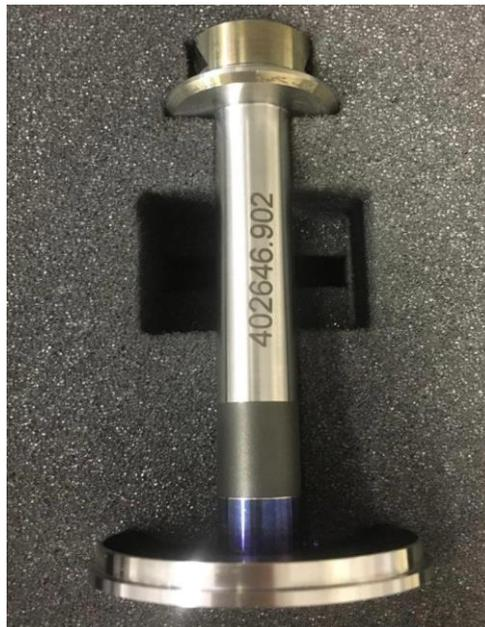
**Figura 11** - Geometria Concentric Cylinders.
