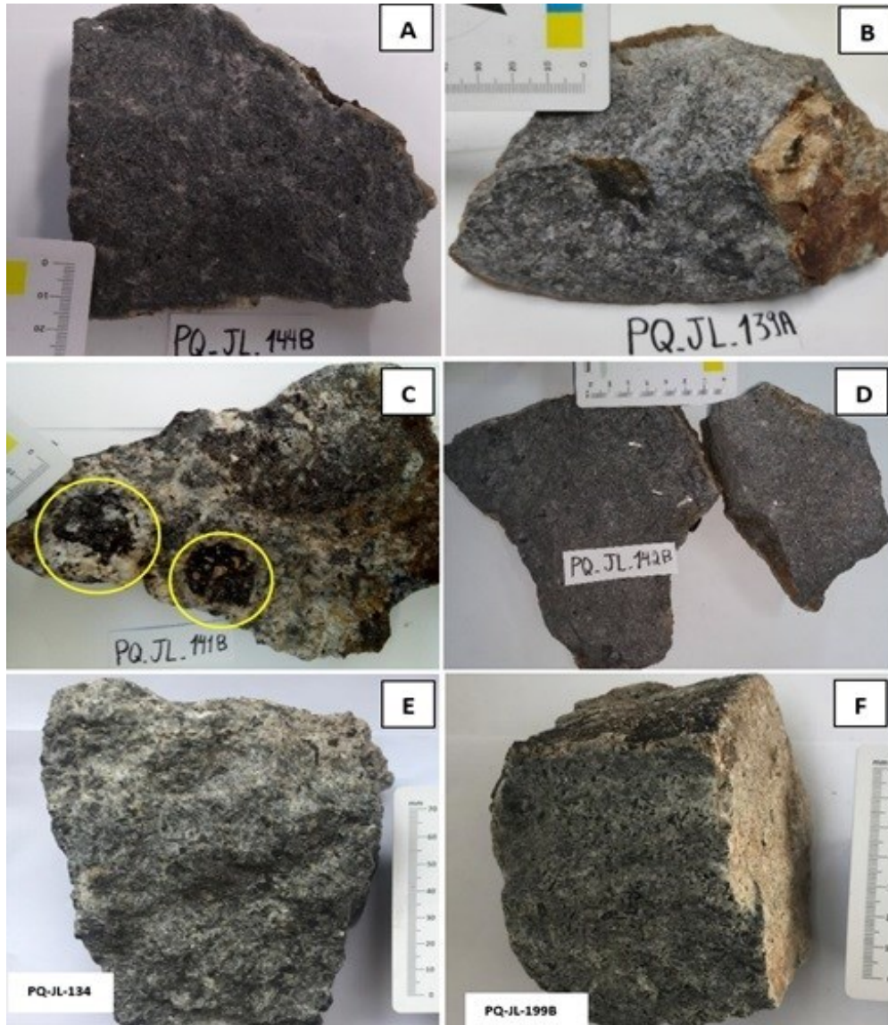
Figure 8. The image display all the lithologies observed in the field: A: Porphyritic phonolite, B: Trachyte, C: Alkali syenite with inclusions of mesocratic monzosyenite (marked by yellow circles); D: Alkali syenite with nepheline, E: Nepheline syenite and F: Alkali syenite with magnetite.
