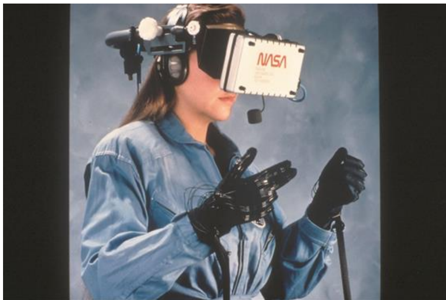
Figura 4 –. The Virtual Interface Environment Workstation (VIEW)
