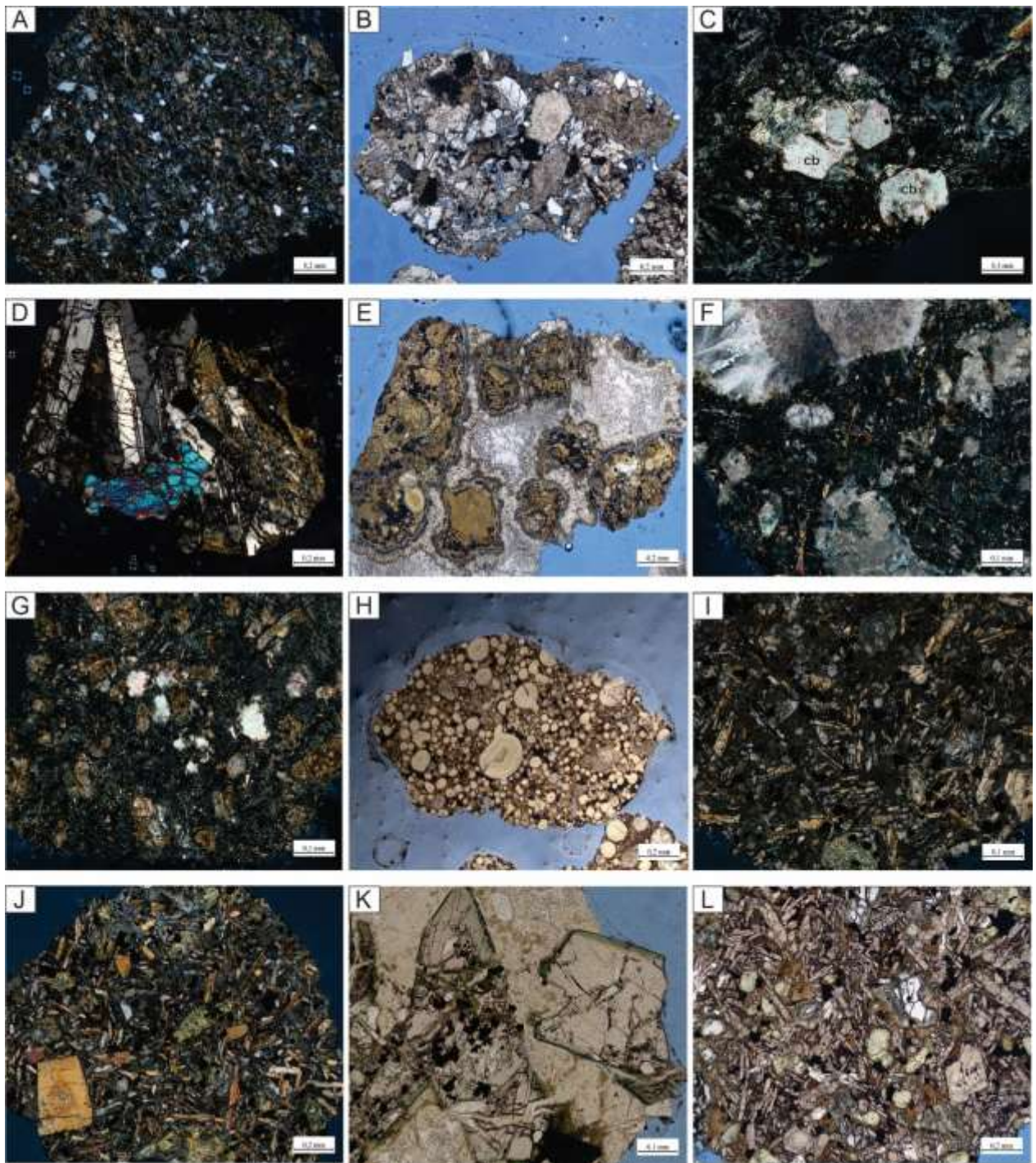
Figure 12. Photomicrographs of drill cutting samples from EG1, EG2 and EG3 wells. A) tuffaceous sandstone 1A-A with angular to subangular crystalloclasts (cross-polarized light); B) medium-welded lapilli tuff 1A-B (plane-polarized light); C) pseudomorphs megacrysts in basaltic scoria lithoclast (1A-C). Original mineral was replaced by carbonate (cb) (cross-polarized light); D) altered diabase intrusion in 1B-A sample (cross-polarized light); E) basaltic scoria lithoclasts in 2A-A lapilli tuff (plane-polarized light); F) amygdaloidal basalt lithoclast in 2A-A lapilli tuff (cross-polarized light); G) porphyritic basalt with carbonate-filled amygdales (2A-B) (cross-
