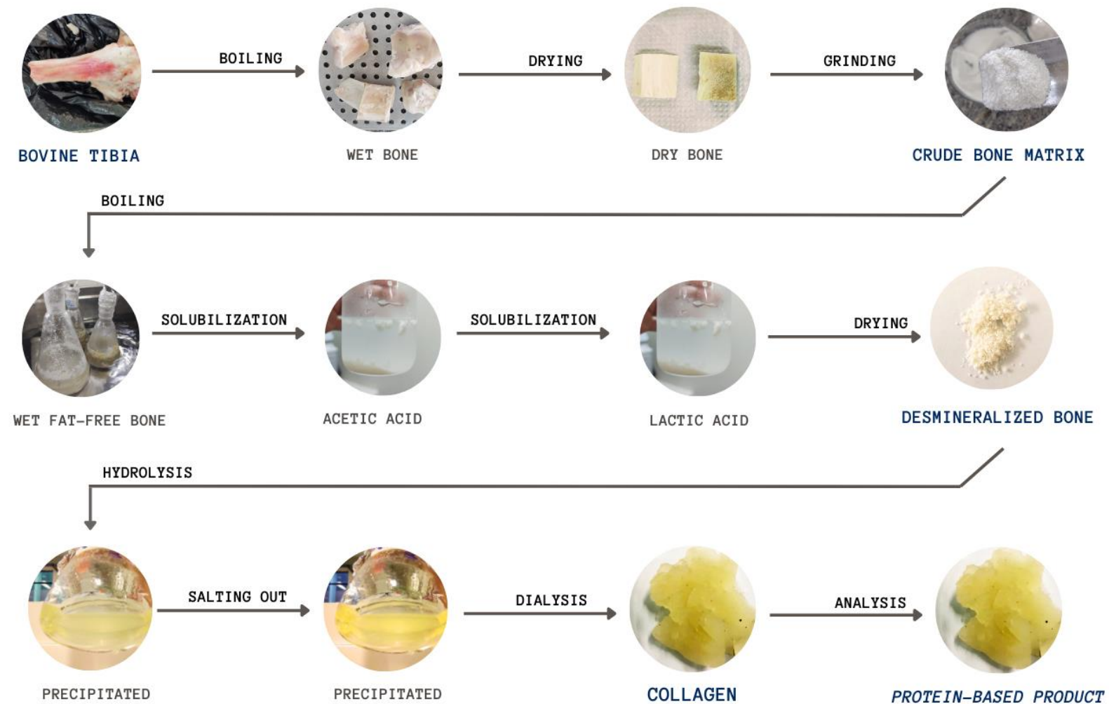
Figure 6.1 - Illustration of the bone processing, demineralization, and collagen obtained process from bovine tibia, exploring the use of bone waste for the protein-based product value chain.
